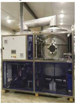
The use of a vacuum system in the installation allows the boiling process to be achieved for liquids at a temperature significantly lower than in normal atmospheric pressure conditions (boiling begins when the liquid reaches 30°C). This can reduce the energy needed for a high boiling point condition and decrease the amount of water consumption as evaporated water can return to the process.
